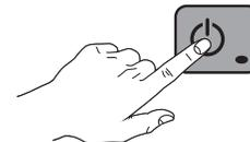
The indicator light of the ON/OFF button “A” (Figure 14) comes on, indicating that the dishwasher is powered and that water is being introduced and heated.
