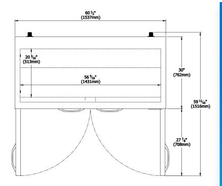
2 Doors Capacity 16.7 Cu.Ft. **Shelves** Refrigerant R-290 Temperature 33°F ~ 39°F Range Easy Sliding Maintenance Condensing Unit 9.8 ft long (3m) flexible three Connection wire cord with modeled plug HP 1/4 HP 115V/60Hz Voltage 4.7 **Amps** NEMA 5-15 **NEMA** Config.
